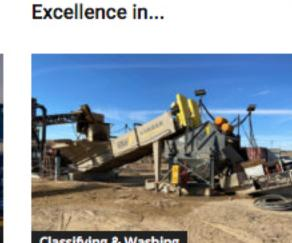
EIW's Eagle+ Dewatering Screen Reduces Moisture Content in Precision Aggregate's
