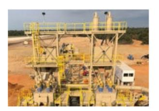
AZFAB Introduces QUAD Attrition Mill Classifying & Washing AZFAB LLC. AZFAB QUAD Attrition Mills were designed to scrub sand particles against
