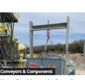
Dings Co. Magnetic Group's Overhead Stationary Electromagnets are Made in the...
