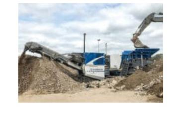
Crushing & Accessories Kleemann With the market launch of the new MOBICAT MC 110(i) EVO2, Kleemann presents a mobile jaw crushing plant of the new generation. The further...
