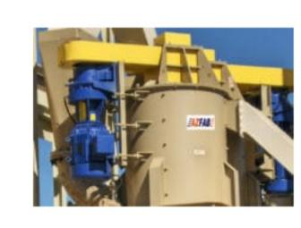
AZFAB Vertical Durability Cell provides the scrubbing power necessary to liberate clays through attrition. Our Vertical Durability Cell can add years
