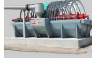
PHOENIX/KISA Bucket Wheel is Designed for the capture, de-sliming and dewatering of granular solids including construction aggregate (sand &
