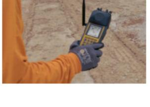
Blasting & Drilling Dyno Nobel Differential GPS (DGPS) is the first ever tagging and hole identification method using Differential Global Position System. High Accuracy DGPS (Differential Global Positioning System) The DGPS...
