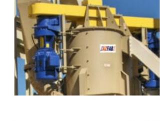
Classifying & Washing AZFAB LLC. AZFAB Vertical Durability Cell provides the scrubbing power necessary to liberate clays through attrition. Our Vertical Durability Cell can add years
