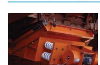
General Kinematics PARA-MOUNT II® Vibratory Feeders
