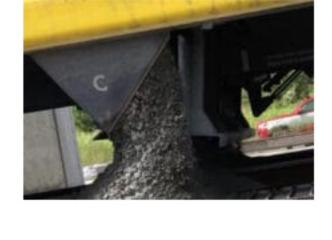
Recurring issues, like spillage at load zones, can create operational inefficiencies from product loss and labor costs. At this location, large lump spillage had...
