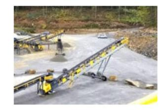
Transfer Conveyors and Radial Stackers from Kemper Equipment
