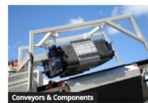
Dings Company's Magnetic Separators Remove Tramp Iron
