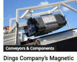
Separators Remove Tramp Iron
